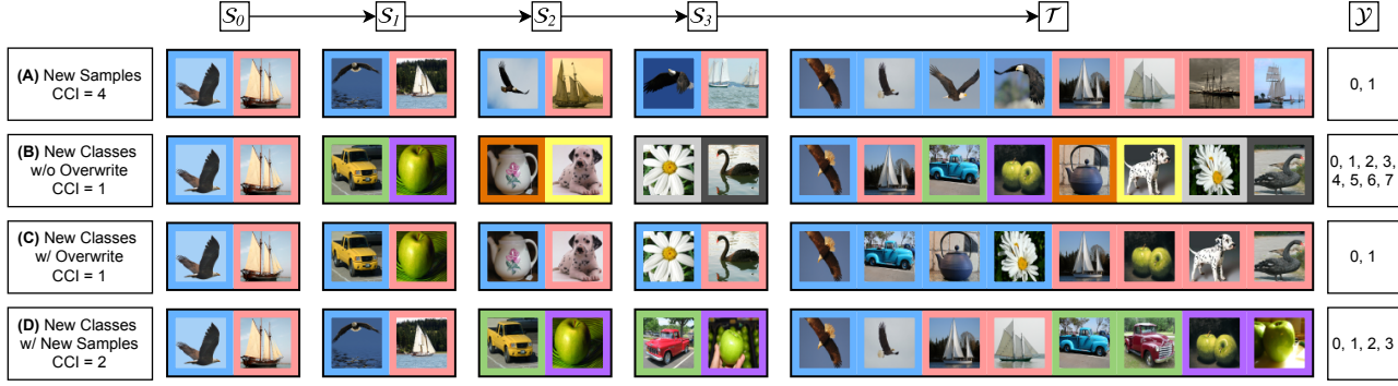
Figure 2: Visual representation of the four continual few-shot task types. Each row corresponds to a task with Number of Support Sets, NSS=4 , and a defined Class-Change Interval (CCI). Given a sequence of support sets, \mathcal{S}_n , the aim is to correctly classify samples in the target set, \mathcal{T} . Colored frames correspond to the associated support set labels.
